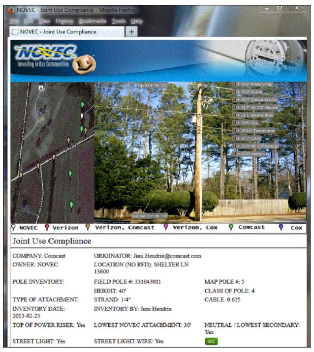
Figure 22: 3rd Party Attachment Compliance Prototype
